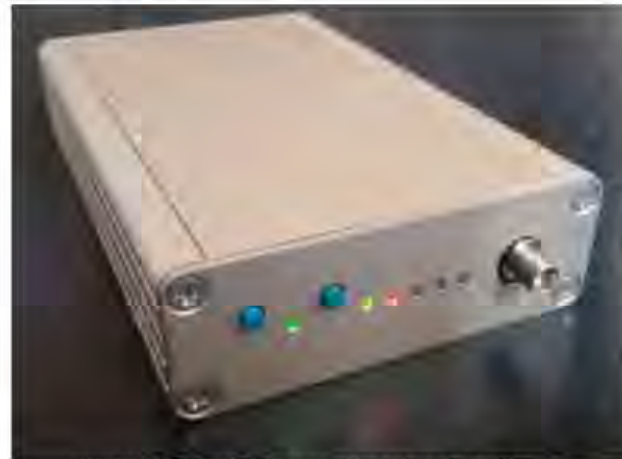
(U//FOUO) HackRF One with optional enclosure
